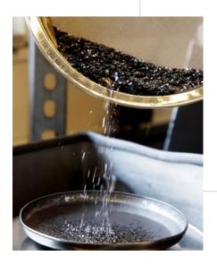
AMG's proprietary V-CYCLE<sup>™</sup> roasting and pyrometallurgical metal recovery process delivers substantial commercial value and environmental risk elimination for refinery partners. By responsibly recycling spent catalysts, we reclaim valuable metals, transforming them into ferrovanadium and other alloys for the steel industry.
