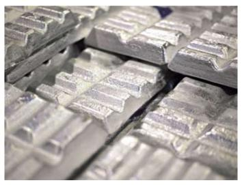
AMG - typical master alloys in ingot form
