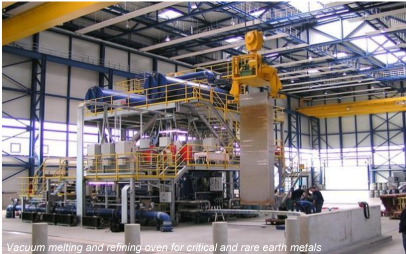
Vacuum melting and refining oven for critical and rare earth metals
